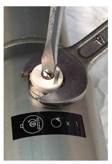
When our pumps leave our factory the air bleed screw cap is always closed. It is therefore important for this to be open when the pump is mounted.
